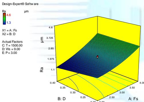
Fig. 5 Effect of the feeding speed and duty factor on the SR
