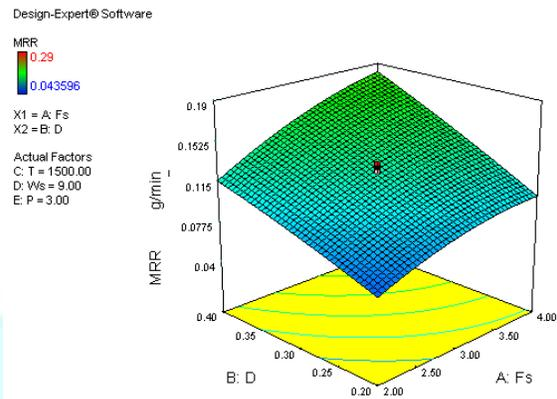
Fig.6 Effect of feeding speed on MRR at various duty factor
