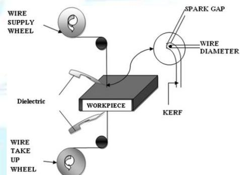
Fig. 1 A schematic of an WEDM
