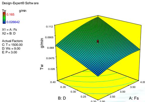
Fig. 4 Effect of the feeding speed on the TW at various duty factor
