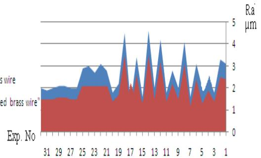
Fig. 11 shows the SR values in the case of using Plane brass wire and in the case of using Nano-coated brass wire
