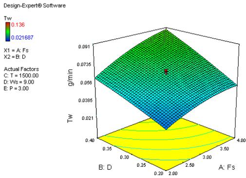
Fig.8 Effect of the feeding speed on the TW at various duty factor
