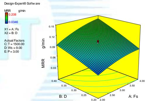
Fig. 3 Effect of feeding speed on MRR at various duty factor
