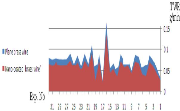
Fig . 9 shows the TW values in the case of using Plane brass wire and in the case of using Nano-coated brass wire
