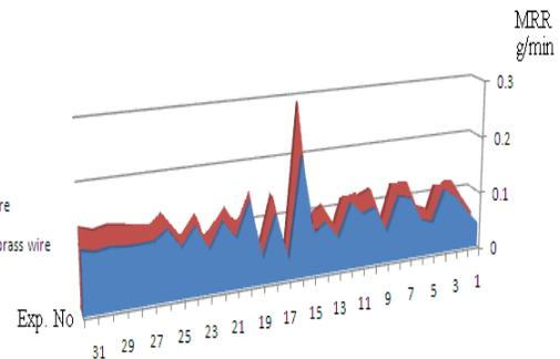
Fig. 7 shows the MRR values in the case of using Plane brass wire and in the case of using Nano-coated brass wire.
