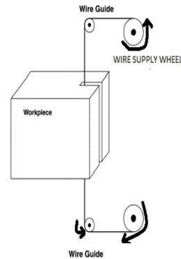
Fig. 2 Schematic of wire-EDM process
