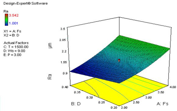
Fig. 10 Effect of the feeding speed and duty factor on the SR
